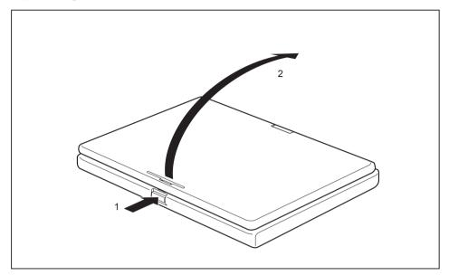
▶ Press the release button (1), and unfold the LCD screen upwards (2).
